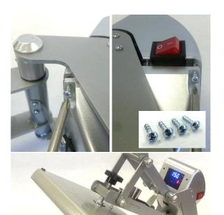
Install top half of Controller Housing and secure by screwing in 4x #6 x ½" Screws using #2 Phillips Screwdriver
