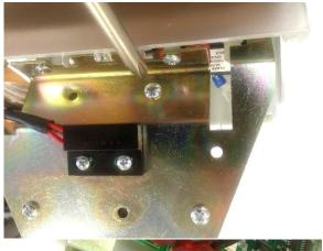
Unscrew old TRIAC using #2 Phillips Screwdriver and remove from bracket
