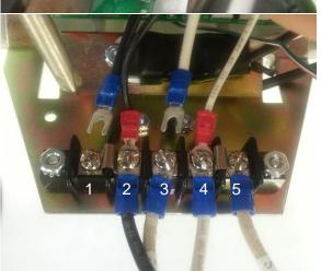
Unscrew and disconnect old TRIAC wires from terminal strip as shown:
